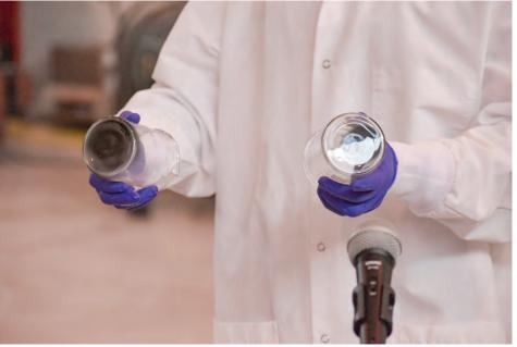
WSU Graduate student Harrison Yang showing the carbon intensity between traditional fossil-based jet fuel (left) and a 50% blend SAF (right) during a demonstration on March 28, 2023. The beaker on the left with traditional fossil-based jet fuel has more soot or carbon residue when burned than the SAF blend. Lynnwood Times | Mario Lotmore.
