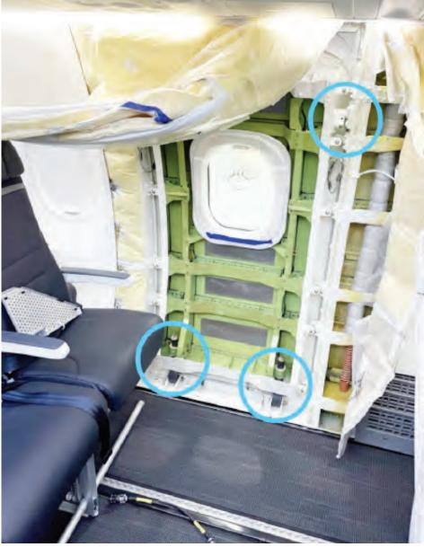
Photo showing the left MED plug immediately before interior restoration and the circles show the three locations without the retaining bolts, two vertical movement arrestor bolts and the forward upper guide track bolt. The aft upper guide track is covered with insulation and cannot be seen in the photo. (Source: Boeing. Image Copyright © Boeing. Reproduced with permission.). SOURCE: NTSB Preliminary findings report of Alaska Airline flight 1282.
